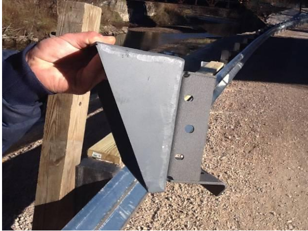
Fabricated housing for angling camera down
